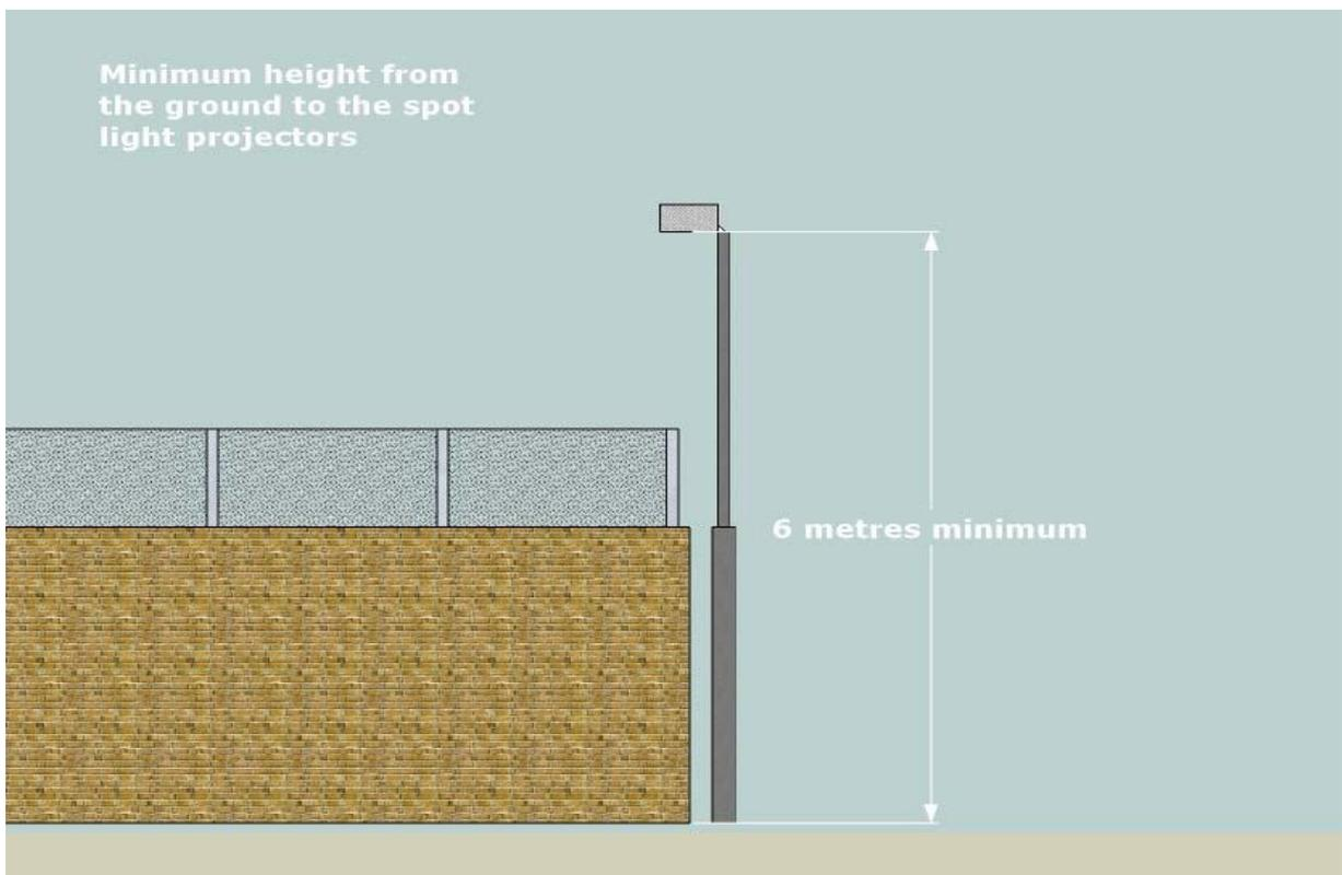
As for the new facilities it is suggested they have a minimum height from the ground to the inferior part of the light projectors of 8 metres if they are installed inside the court considering the vertical projection of the court side walls. Different heights for lighting can be installed for lights installed outside the court walls
